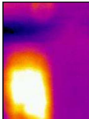
Proof that MACo's new thermal imaging camera, a HotShot LT from Electrophysics, can inspect areas more effectively than the human eye is shown in the above images recently made by MACo Loss Control Specialist Fred Hansen. The picture on the left shows a normal view of a building's electrical box, while the picture on the right is an infrared view of the same box displaying a thermal hotspot (in white). The temperature variation was caused by a minor mechanical issue that was repaired.
